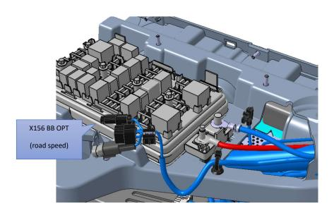
If your device does not recognize road speed signal. Check that the parameter is set correctly.
